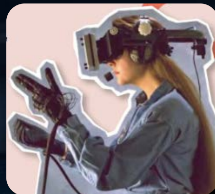
Rys. 6. Zestaw HMD – Head Mounted Display i cyberrękawice z Ames Research Center NASA [4]
